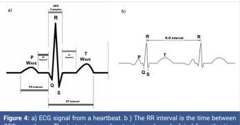
QRS complexes. The instantaneous heart rate can be calculated from the time between any two QRS complexes.
