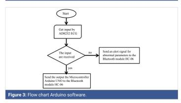
whether all three inputs are given properly. If someone of the inputs is not detected well, the system send a warning; if all inputs are detected, the software send the signal thought the Bluetooth module HC-06 at the Android application to process cardiac parameters.
